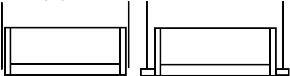
The above diagram shows the ropes going straight up. To achieve this look you will more than likely have to have special blocking installed in your ceiling joists. Please see table on the next page that shows swing hole spacing for blocking. This is generally not an option on an older home unless you have access to the ceiling joists above the finished ceiling, or unless you have exposed beams.
