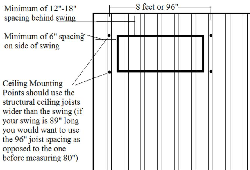
\*\* The mounting points into the ceiling joists need to be wider than the length of the swing to keep the ropes from rubbing on the handrails.
