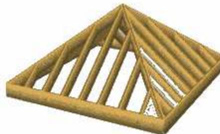
The hip roof installations require more planning on which particular joists you will use and locations or the relative ceiling joists going the opposite direction if trying to place the swing in the corner.
