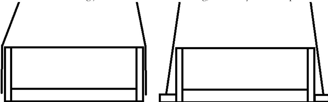
The above diagram shows how the ropes will look if the mounting points in the ceiling joists are narrower than the swing. This is not recommended as it will limit the swinging motion and may cause the rope to rub on the side of your swing and could potentially rub the finish off of your swing on the sides.
